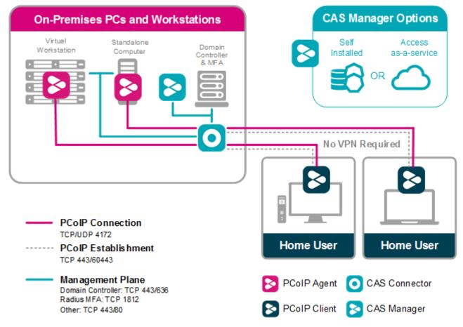
Teradici recommends using TCP 60443 for internal connections. It is not mandatory for TCP 60443 to be opened to the public network.
