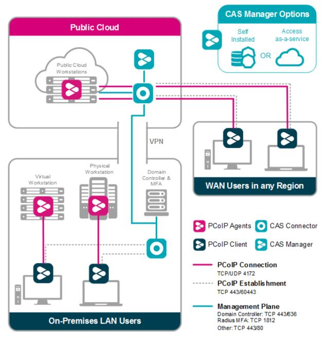
Teradici recommends using TCP 60443 for internal connections. It is not mandatory for TCP 60443 to be opened to the public network.
