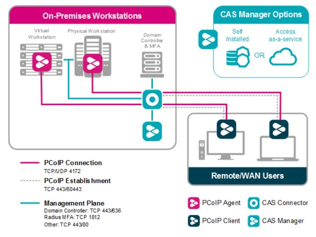
Teradici recommends using TCP 60443 for internal connections. It is not mandatory for TCP 60443 to be opened to the public network.
