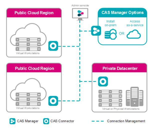
In addition to managing cloud compute costs, CAS Manager handles user entitlement, authentication (including RADIUS-compatible multifactor authentication (MFA)) and brokering of connections during PCoIP session establishment. The CAS Connector enables external users to access their remote desktops without the complexity of endpoint VPN's.
